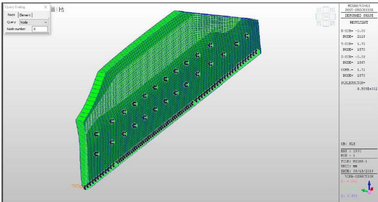
**Figure 6: Lateral Displacement of Retaining Wall with Tie Back Anchors under SLS Condition**
