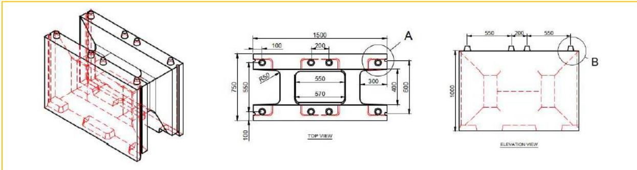
**Figure 1: Typical RASBlox Dimensions**
