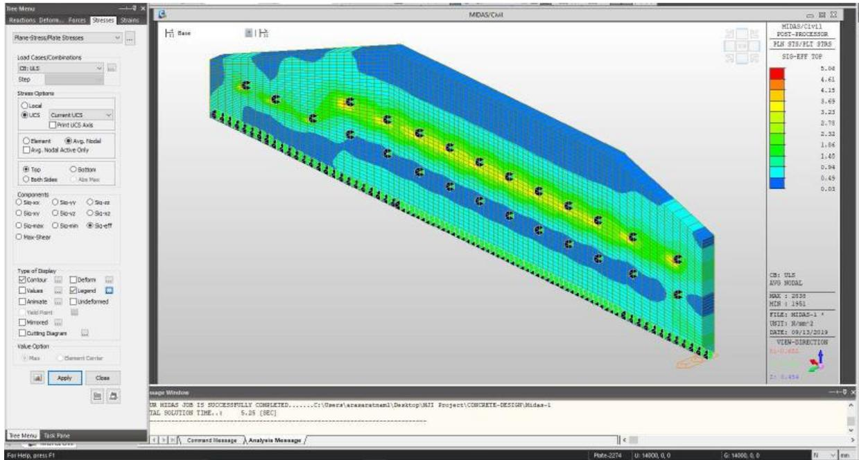
**Figure 7: Effective Stress Contours within Retaining Wall with Tie Back Anchors under ULS Condition**
