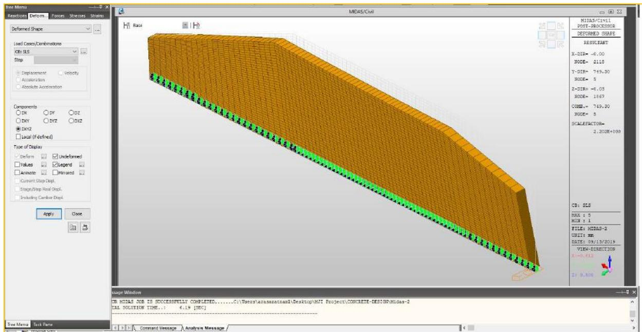
**Figure 3: Lateral Displacement at the tip of the Retaining Wall**
