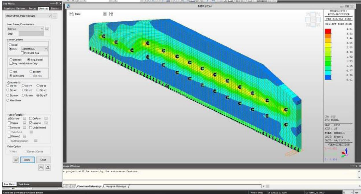
**Figure 8: Effective Stress Contours within Retaining Wall with Tie Back Anchors under SLS Condition**
