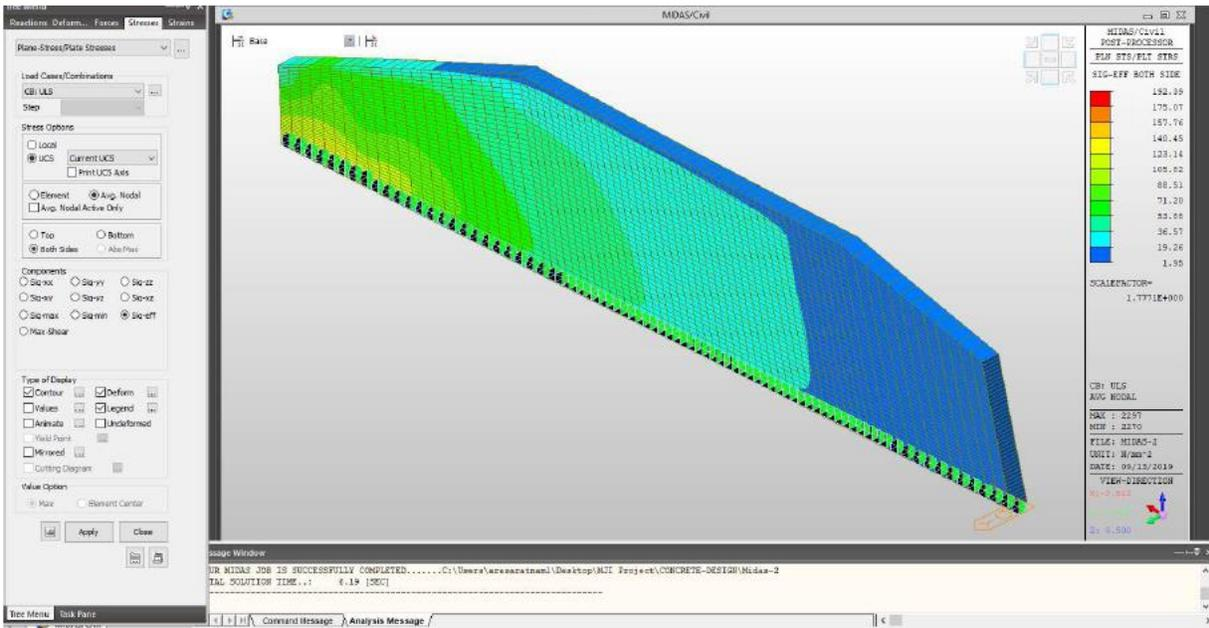
Figure 4: Effective Stress Contours within Wall under ULS Condition
