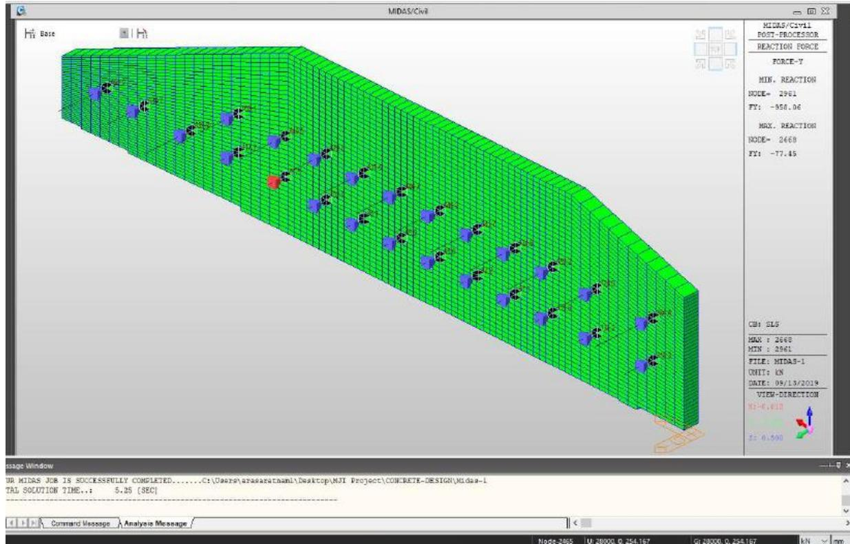
Figure 9: Forces on Tie Backs under ULS Condition
