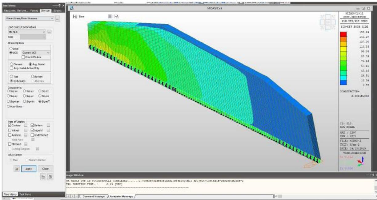
Figure 5: Effective Stress Contours within Wall under SLS Condition
